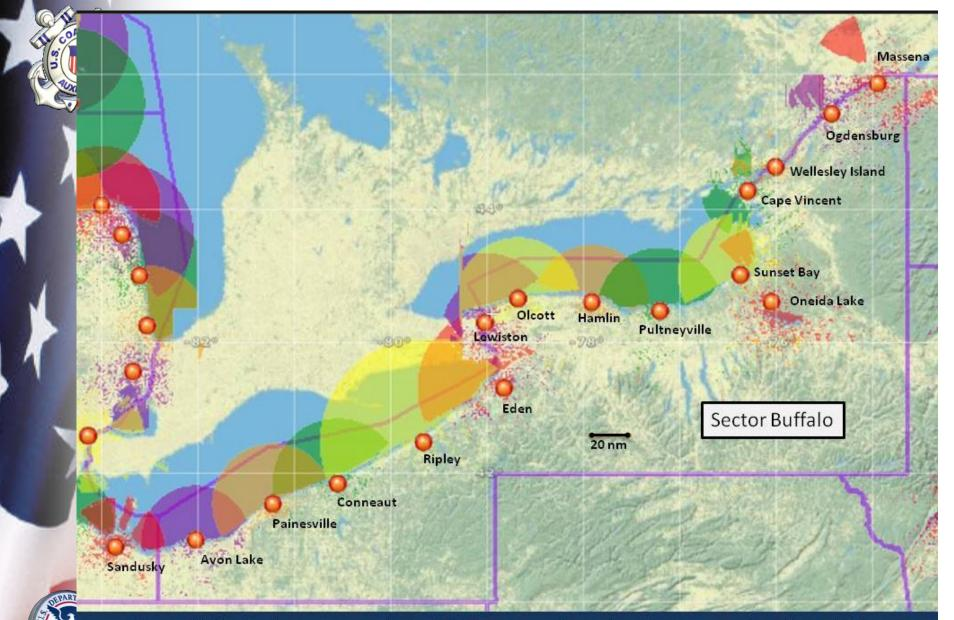
Rescue21 Regional coverage analysis of VHF receive antenna based on geographical line-of-sight. System requirement: At least 20 nm offshore for a 1 watt VHF-FM Ch 16 signal transmitted form two meters above water surface.
